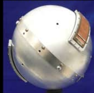
Pod structure showing dual-band UHF antennas
