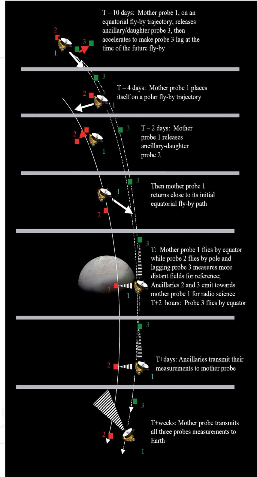
T – 10 days: Mother probe 1, on an equatorial fly-by trajectory, releases ancillary/daughter probe 3, then accelerates to make probe 3 lag at the time of the future fly-by
