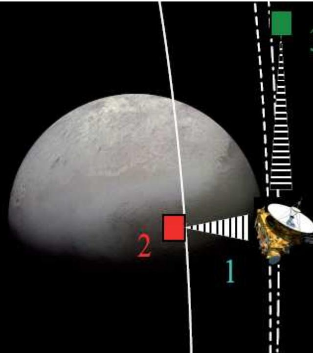
T: Mother probe 1 flies by equator while probe 2 flies by pole and lagging probe 3 measures more distant fields for reference;
